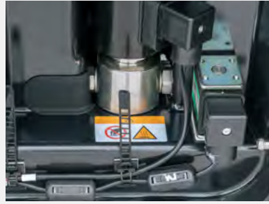
This label warns you of the existence of the high temperature hazard near its proximity.
