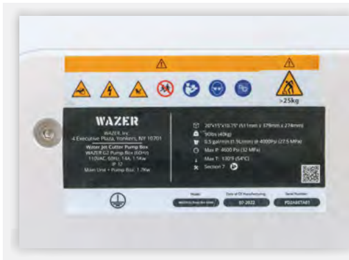
This label warns you of the operation, maintenance, and repair hazards of the WAZER Pump Box.
