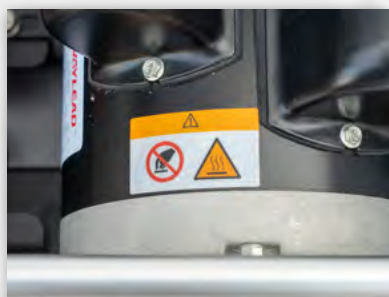
This label warns you of the existence of the high temperature hazard near its proximity. Caution is advised to avoid injury.
