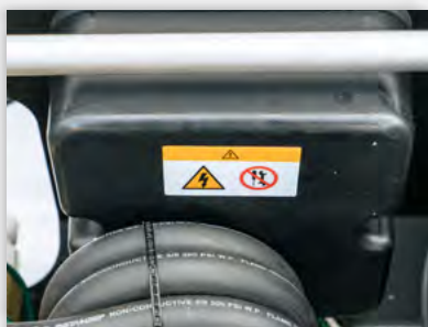
This label warns you of the residual hazards inside the WAZER Pump Box Electrical Enclosure and instructs for it to not be opened up.
